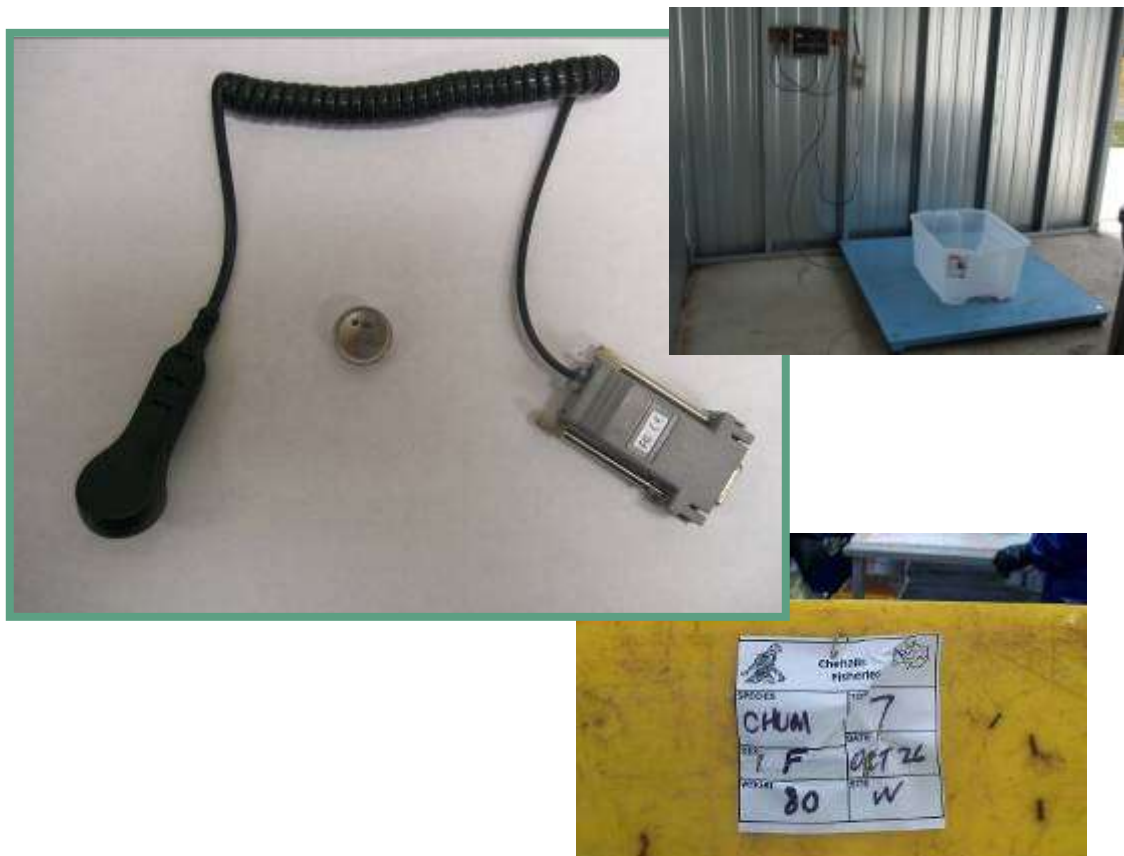
Figure 27. Temperature logger used in field cooling trials, a digital tote scale, and a simple but important tote tag
